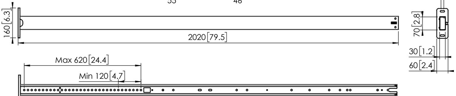
If needed, for shorter lengths cut off this part from the bottom to the desired length. (holes for mounting the foot)
