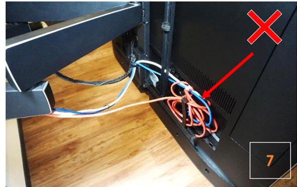
The TV interface of the Motion(Sound)Mount is fixed to the back of the TV. This side will not be seen and is there for suitable for hiding the remnant cable. The down side is that the back side of the TV is limited to how much remnant cables can be routed here.
