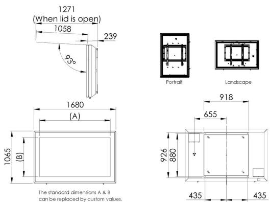
The standard dimensions A & B can be replaced by custom values.
