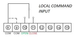
LOCAL COMMAND INPUT: allows the LOCAL command of the motor or system. The type of command is IMPULSIVE and the contacts are voltage-free. To stop the engine give an inverse command respect to the one in progress (ex: if OPEN = CLOSE). Timed command. Multiple buttons can be connected in parallel. Recommended cable for connection: 3x0.25 mm or 3x0.22 mm.
