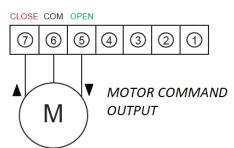
**MOTOR OUTPUT CONNECTION:** connect the cable OPEN of the motor to the clamp 5 (motor wire brown), the cable CLOSE to the clamp 7 (motor wire black) and the COMMON motor cable to the clamp 6 (motor wire blue). Motor wire yellow/green will not be connected. Power charge allowed: MAX 500 W. Cable recommended for the connection: 3 x 0,75 mm.
