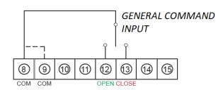
GENERAL COMMAND INPUT: allows the GENERAL command of the engine or system. The type of command is IMPULSIVE and the contacts are voltage-free. To stop the engine give an inverse command respect to the one in course (ex: if OPEN = CLOSE). Timed command. It's possible to connect several buttons in parallel with each other. Cable recommended for connection: 3x0.25 mm or 3x0.22 mm.
