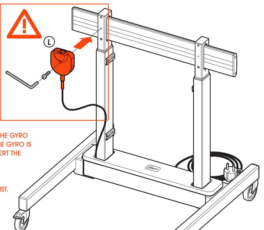
**WARNING: THE LIFT DOES NOT FUNCTION IF THE GYRO IS NOT MOUNTED CORRECTLY. MAKE SURE THE GYRO IS MOUNTED FIRMLY TO THE COLUMN AND INSERT THE CONNECTOR INTO THE CONTROL BOX.**
