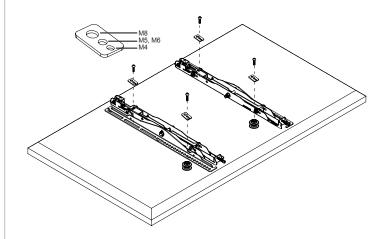
Universal Washers are designed to accommodate the various M4, M5, M6 and M8 hole sizes required by flat-panels.
