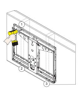
Drill a pilot hole in each of the three (3) marks with a power drill and a M6 or 1/4" drill bit.
