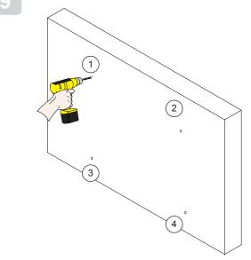
Drill a pilot hole in each of the four (4) mark areas with a 3/8" masonry drill bit.
