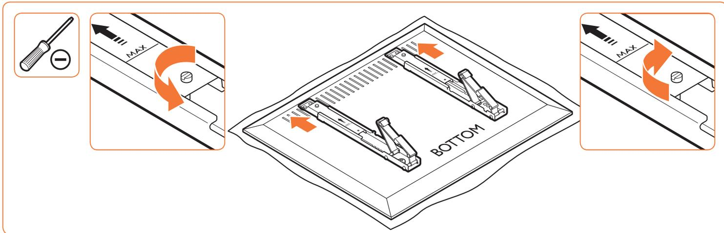
• **Depending on the screen size: adapt the strip length to fit the mounting hole pattern. Do not extend any further than 'MAX'.**
