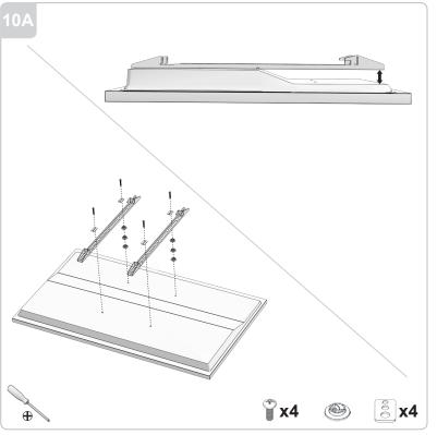
Once the correct pitch and depth screws are pulled from the hardware pack supplied, secure the two brackets to the rear of the display with the proper screws and plate washer holes. Plastic spacers are also supplied in case you need additional clearance between the bracket and the rear of the display. NOTE: Do not over tighten the screws.
