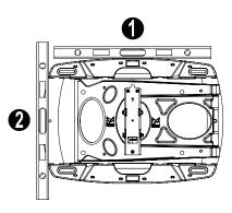
Re-install the front wall arm plate to the arm with the three M5 flat head screws you set aside earlier. Confirm screws are fully seated and tight.
