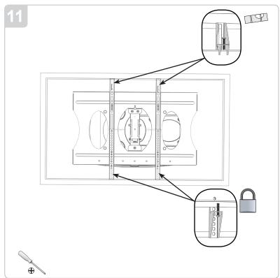
Center the display horizontally on the plate and check the display is level on the mount. To adjust level, adjust the left or right top screw to achieve desired level of the display. Once level, secure the lower left and right security screws on the bracket to "fix" the mount to the wall mount.
