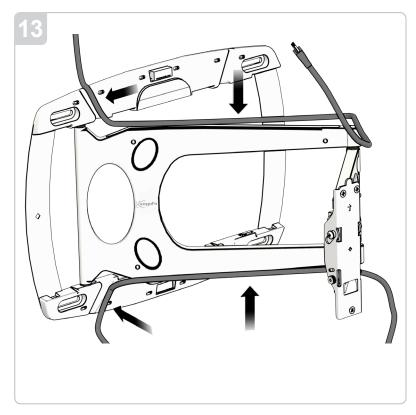
We recommend where possible that the power and signal cables be run separately through the mount until mating at the display plug in points to minimize possible "cross talk" interference. With the covers removed, cable can be run inside the upper and lower main arm and through the slots behind the plastic beauty covers.
