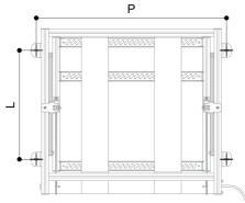
Mark these measures onto the ceiling, in the required position, taking care to keep the squareness between the four points.
