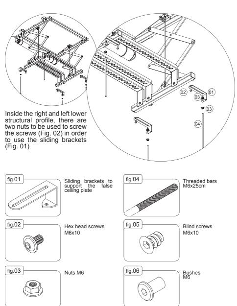
The sliding brackets (fig. 01) have to be positioned in the suitable point in order to fix correctly the false ceiling plate.
