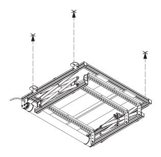
After having fixed the lift to the ceiling, please remove the panels from the lift structure.
