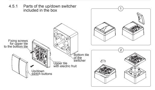
Fig. 1 Without using screwdrivers, remove the up/down buttons.
