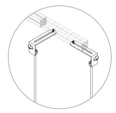
After fixing the threaded bars (fig. 04) and defined the right length, the false ceiling plate can be mounted using two types of screws.
